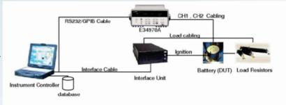
Thermal Battery Test & Measurement Setup
