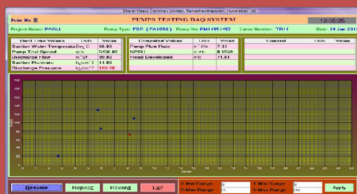
NPSH test for 1% and 3% Head break down
